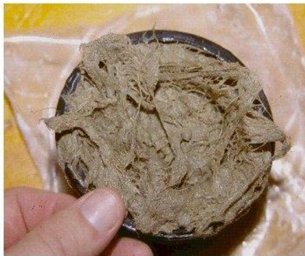
Figure 4. The same tile as in figure 3 after rinsing. Washing out the soil may reveal roots of trees or other vegetation that has entered through perforations. The roots are often fibrous, packed very tight within the drain. Although soil was caught in the root mass, the real cause of the blockage was by roots.
